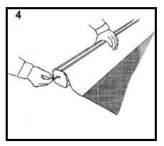
Grip the image and display with your left hand. Remove the locking pin with your right hand.
